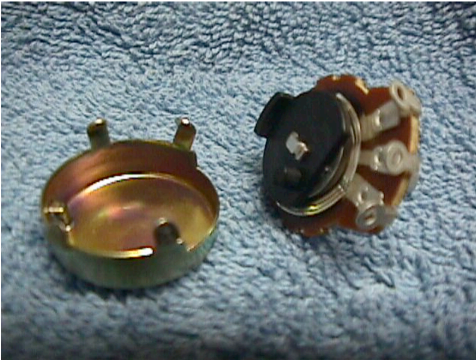
All the fun stuff appears to be inaccessible under that black plastic cover. Actually, that cover performs a couple of very useful functions; it serves to hold the wiper in place, and also interacts with the stop on the case to set the mechanical rotation limits. If you remove the tab on the plastic disk and reassemble the pot, it will now rotate freely 360 degrees. Here's a little better view of the shaft/wafer/wiper assembly.
