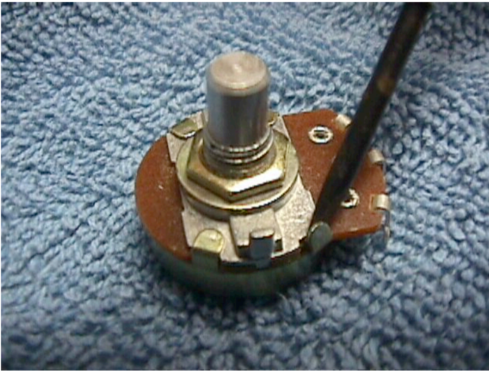
When they're all bent up, you can lift the shaft and phenolic wafer assembly out of the back housing like this.
